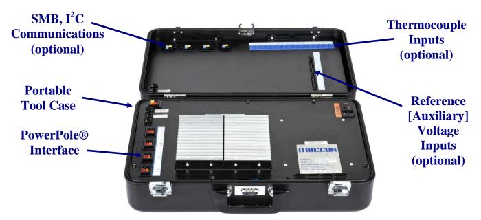
The Model 4400 is supplied as a complete turnkey system with Laptop PC and software. Powered by Maccor's standard test system software and utilizing the same technology found in Maccor's high-precision Series 4000 Automated Test System, the Model 4400 is the perfect portable test system in Maccor's line of high-quality, dependable test systems.
